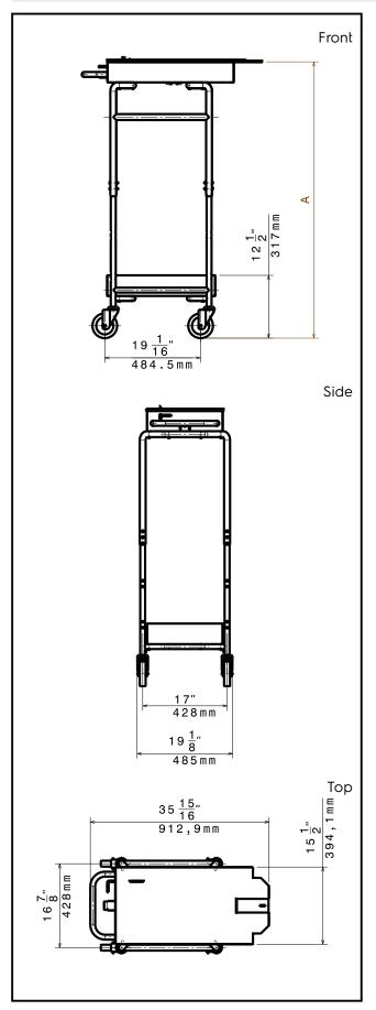
Cooking accessories Trolley for slide-in rack for 6 & 10 GN 1/1 oven and blast chiller freezer
